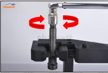
⚠ The tightening torque of the nozzle cap must be installed in accordance with the tightening torque specified in the injector maintenance manual
